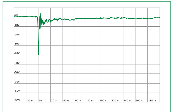
IEC 61000-4-2 -8 kV Contact ESD Clamping Voltage
