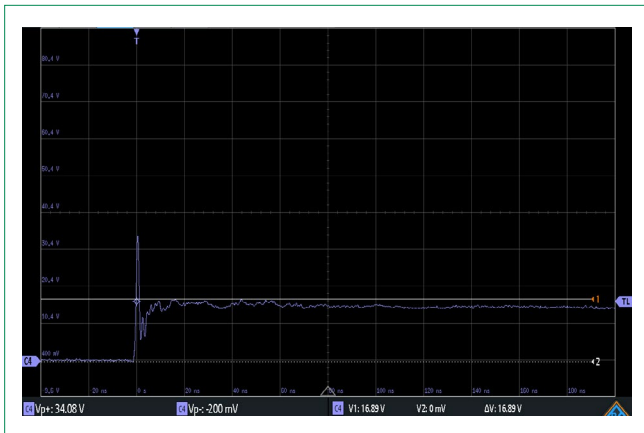
SC1115 IEC 61000 -4-2 +8 kV Contact ESD Clamping Voltage
