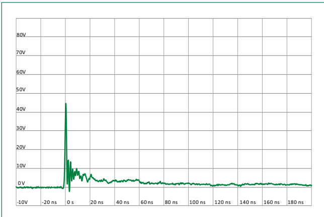
IEC 61000-4-2 +8 kV Contact ESD Clamping Voltage
