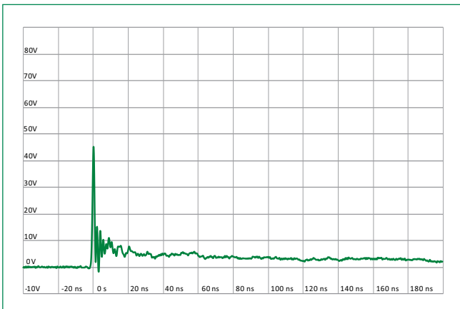
ISO10605 Contact Discharge Plot at +8KV
