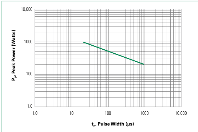
Figure 1. Pulse Rating Curve
