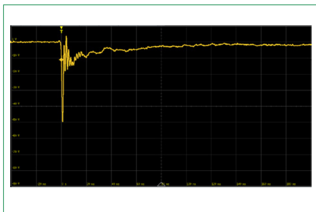
IEC 61000-4-2 -8 kV Contact ESD Clamping Voltage
