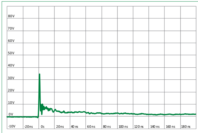
IEC 61000-4-2 +8 kV Contact ESD Clamping Voltage
