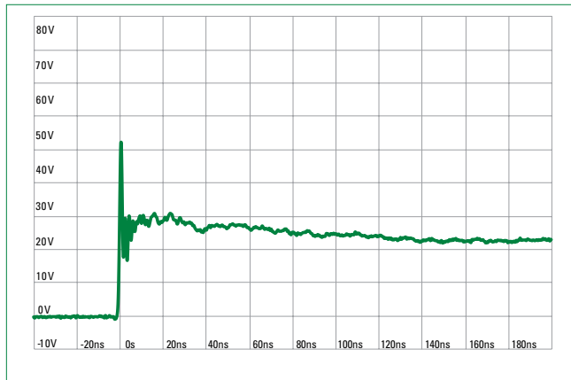
IEC 61000-4-2 +8 kV Contact ESD Clamping Voltage
