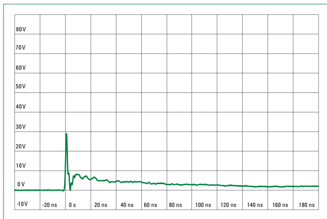
IEC 61000-4-2 +8 kV Contact ESD Clamping Voltage
