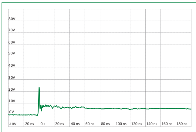
IEC 61000-4-2 +8 kV Contact ESD Clamping Voltage
