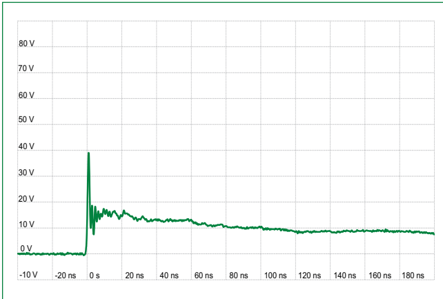
IEC 61000-4-2 +8 kV Contact ESD Clamping Voltage
