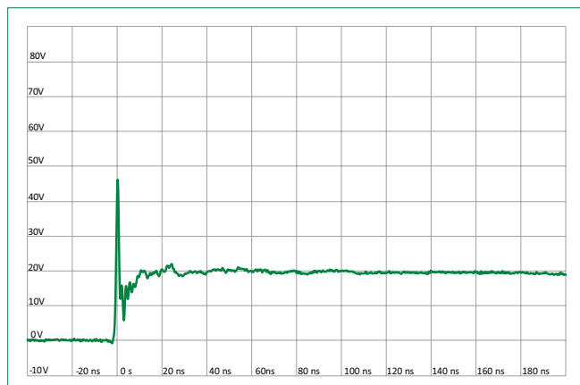
IEC 61000-4-2 +8 kV Contact ESD Clamping Voltage
