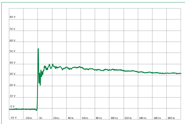
ISO10605 Contact Discharge Plot at +8 kV
