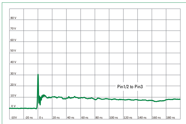
IEC 61000-4-2 +8 kV Contact ESD Clamping Voltage
