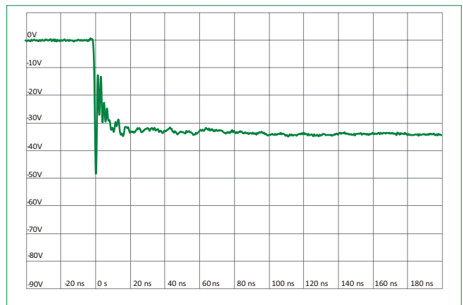
ISO10605 Contact Discharge Plot at -8 kV
