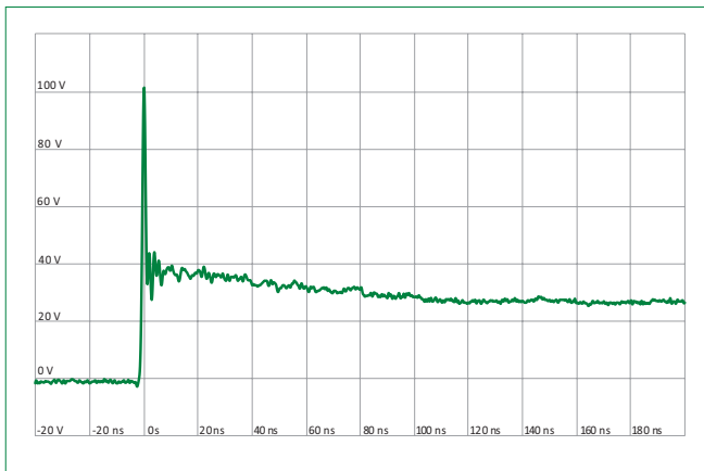
ISO10605 Contact Discharge Plot at +8 kV
