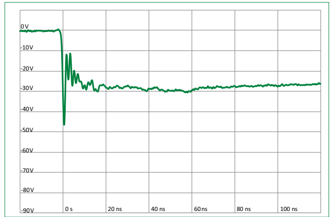
IEC 61000-4-2 -8 kV Contact ESD Clamping Voltage
