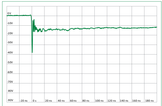
IEC 61000-4-2 -8 kV Contact ESD Clamping Voltage
