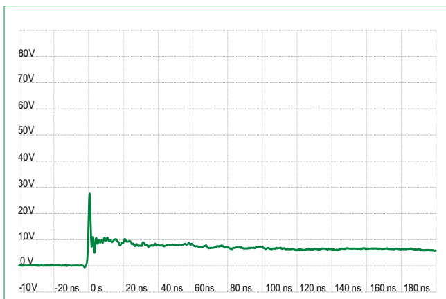
ISO10605 Contact Discharge Plot at +8 kV
