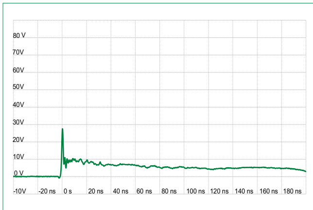
IEC 61000-4-2 +8 kV Contact ESD Clamping Voltage
