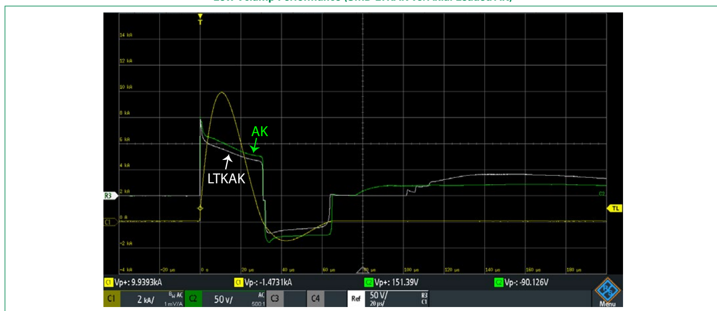
Low V_{CLAMP} Performance (SMD LTKAK vs. Axial Leaded AK)
