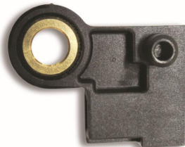
Figure 3: Linear Position Sensor
