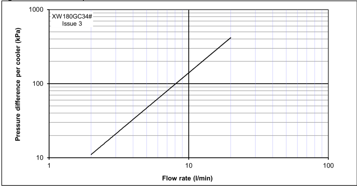
Figure 3 – Pressure drop vs Water flow
