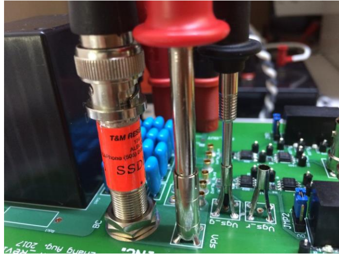
Figure 11. Probe-tip to PCB Interface Connections
