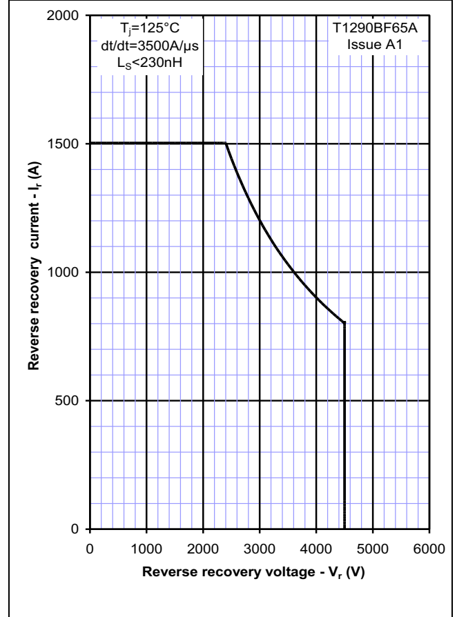
Figure 6 – Safe operating area (Diode)
