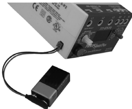
Figure 3: Proper Position of the Battery Cable
