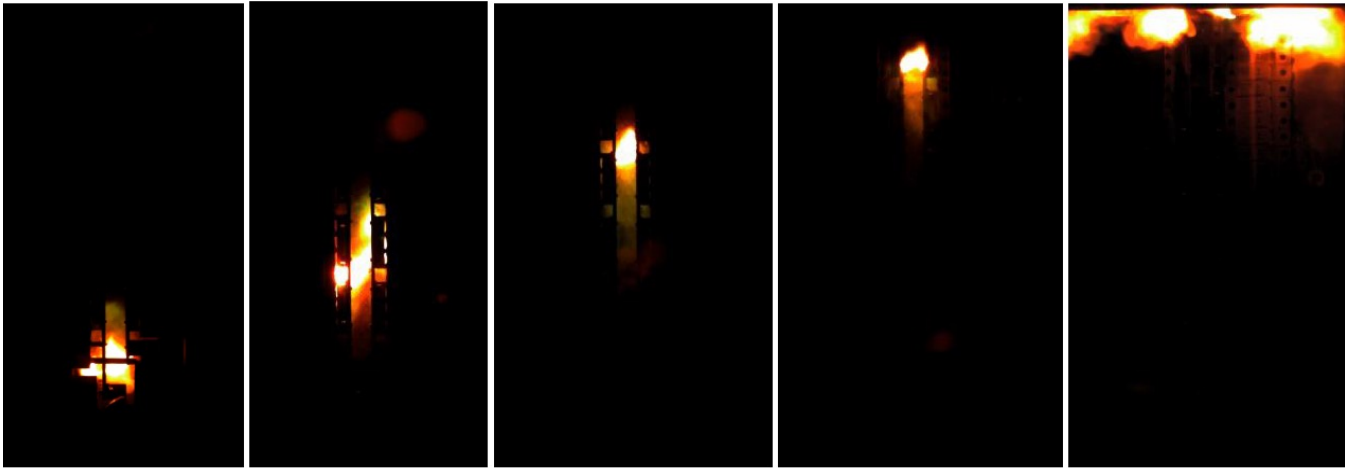
FIGURE 10. Freeze frames from high-speed video with light filter showing short circuit on dc bus with a 1000 A maximum current.
