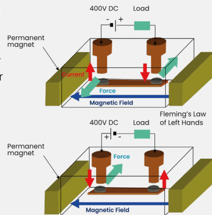
Polarized magnets in relays offer better alignment of the magnetic field lines and arc displacement, leading to superior arc quenching when current flows in the correct direction. Non-polarized magnets are a compromise, providing better alignment than polarized magnets when current is reversed but still inferior to polarized magnets in optimal conditions.
