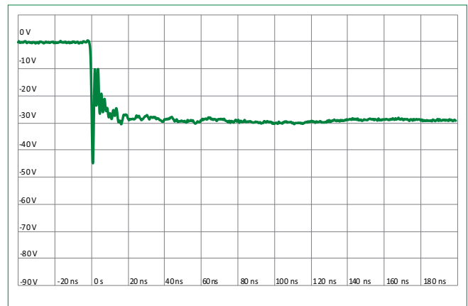
ISO10605 Contact Discharge Plot at -8 kV
