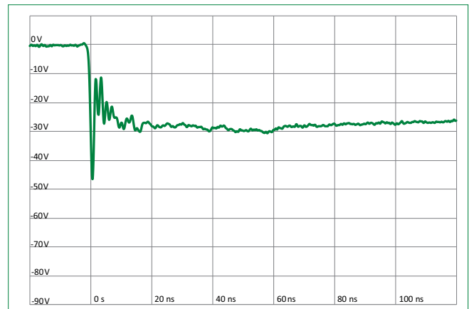
IEC 61000-4-2 -8 kV Contact ESD Clamping Voltage
