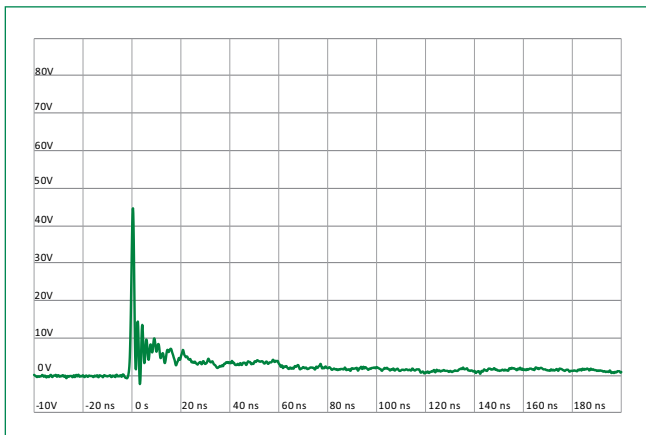
IEC 61000-4-2 +8 kV Contact ESD Clamping Voltage
