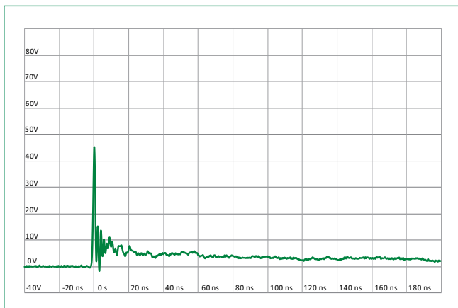
ISO10605 Contact Discharge Plot at +8KV
