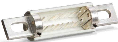
Figure 8. Cut-away of high-speed fuse
