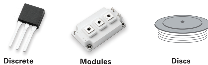
Figure 5. Power semiconductor device packaging
