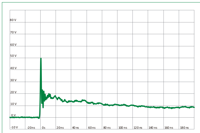
IEC 61000-4-2 +8 kV Contact ESD Clamping Voltage
