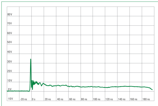
IEC 61000-4-2 +8 kV Contact ESD Clamping Voltage
