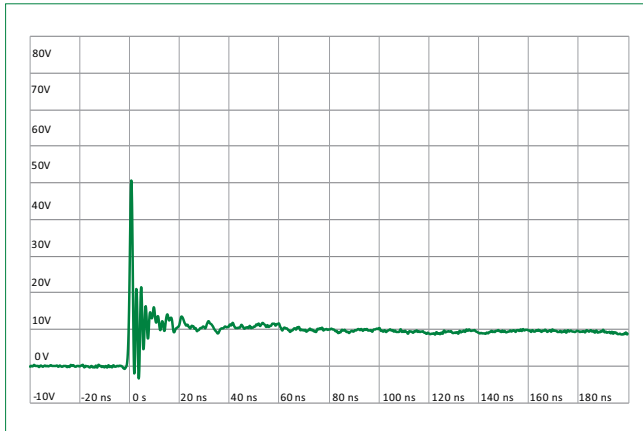
ISO10605 Contact Discharge Plot at +8 kV
