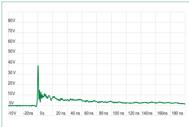
IEC 61000-4-2 +8 kV Contact ESD Clamping Voltage
