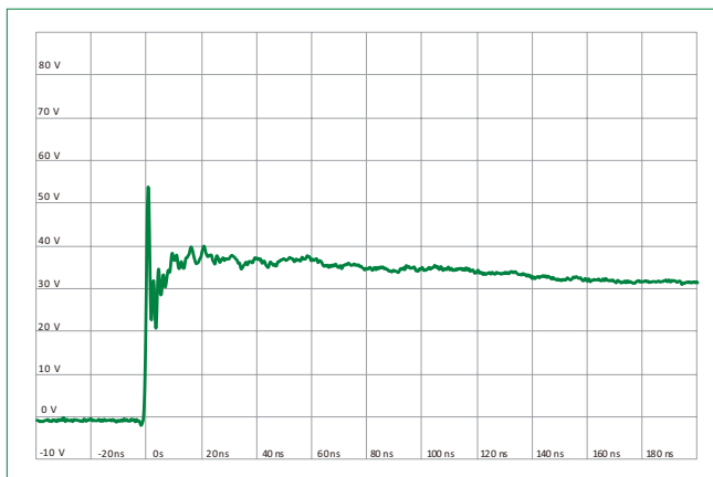
ISO10605 Contact Discharge Plot at +8 kV
