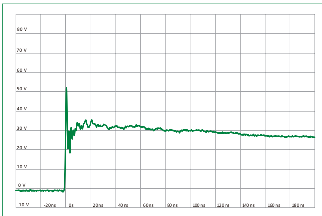
ISO10605 Contact Discharge Plot at +8 kV
