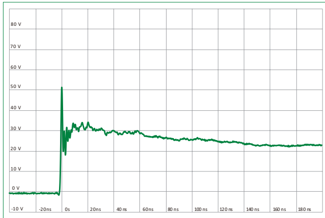
IEC 61000-4-2 +8 kV Contact ESD Clamping Voltage
