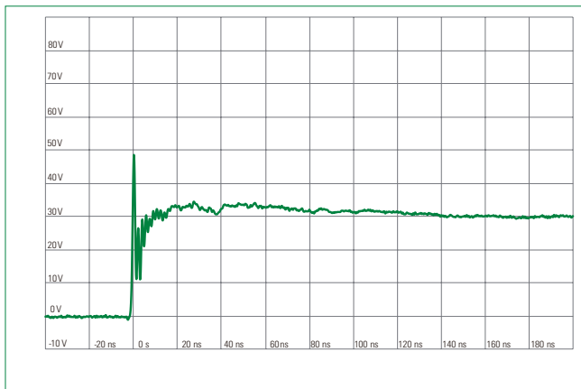
ISO10605 Contact Discharge Plot at +8 kV
