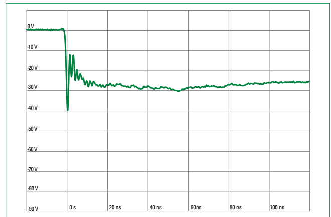
IEC 61000-4-2 -8 kV Contact ESD Clamping Voltage
