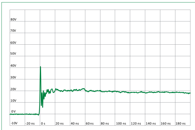
ISO10605 Contact Discharge Plot at +8 kV
