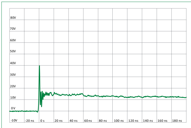
IEC 61000-4-2 +8 kV Contact ESD Clamping Voltage
