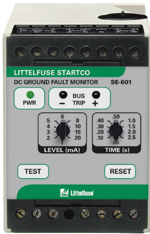
Figure 2. The SE-601 DC Ground-Fault Monitor provides sensitive, fast ground-fault protection with nuisance tripping. Ground-fault current is sensed using an SE-GRM Series Ground-Reference Module—a resistor network that limits ground-fault current to 25 mA. The SE-GRM allows an SE-601 to be connected to systems up to 1200 Vdc and potentially higher.
