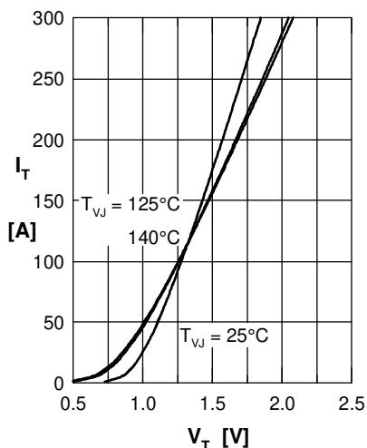
Fig. 1 Forward characteristics
