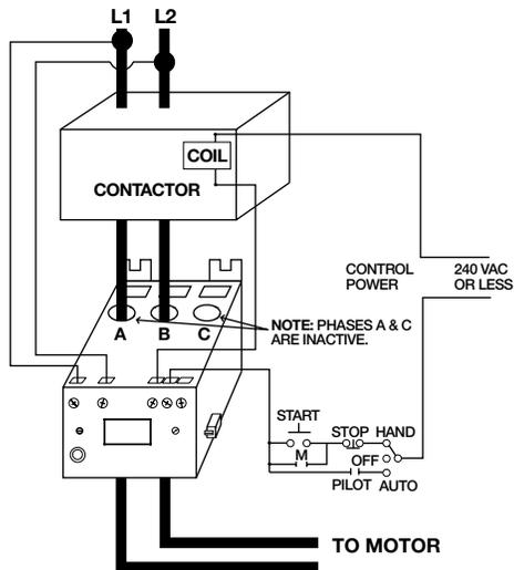
TYPICAL WIRING DIAGRAM FOR MODEL 77C-KW/HP WITH EXTERNAL CT
