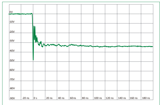
ISO10605 Contact Discharge Plot at -8 kV
