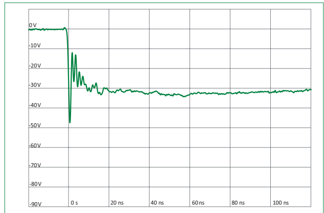
IEC 61000-4-2 -8 kV Contact ESD Clamping Voltage
