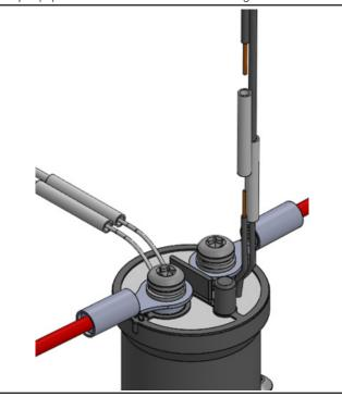
If an Auxiliary Contact is provided, connect the low power Line feed wire to one of the black wires and the low power Load output wire to the remaining black wire. When installing the wires, be sure that a good electrical connection is made. Do not allow any loose strands to short against any equipment and cause electrical damage.
