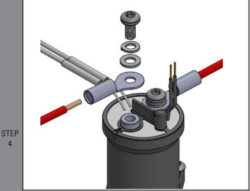
Verify the switched contacts are open, no continuity between terminals "A1" and "A2". Using the hardware that is supplied with the contactor or the recommended fasteners, connect the Line power feed wire to the contactor terminal marked "A1". Connect the Load power output wire to the contactor terminal marked "A2". As with the control wires, be sure that a good electrical connection is made. Do not allow any loose strands to short against any equipment and cause electrical damage.
